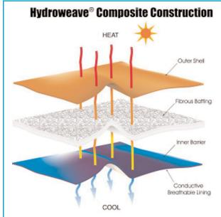
Hydroweave's patented composite construction delivers outstanding cooling performance in a lightweight, versatile product.
