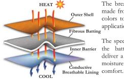
The breathable outer shell can be made from a variety of fabrics and colors to address a wide range of applications.
